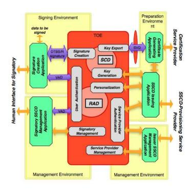
Figure 4: TOE and operational environments with Key Generation and trusted channel to CGA
