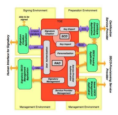
Figure 3: TOE and operational environments with Key Import
