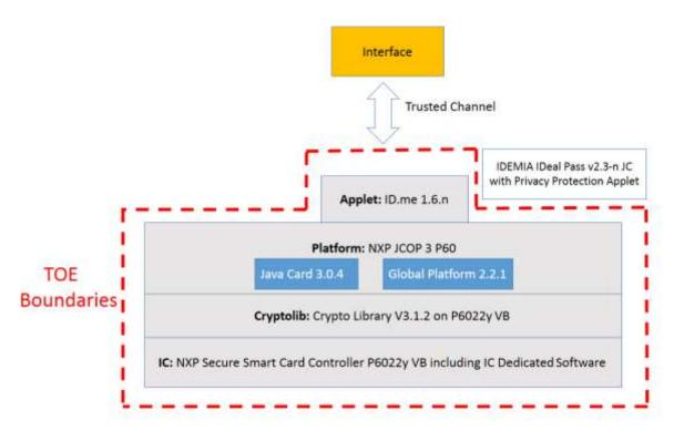
Figure 1: TOE physical scope
