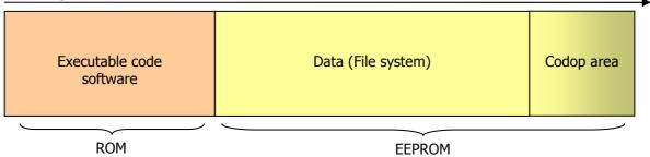
Figure 2 Memory mapping of the TOE
