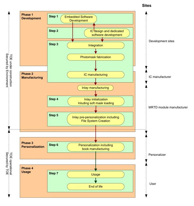
Figure 3: LC1bis: Init on inlay at Gemalto site
