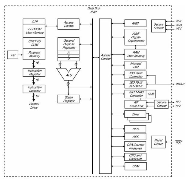
Figure 1: Block Diagram of the AT90SC28880RCFV TOE
