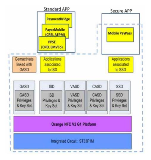
In the previous figure doted lines identify the TOE: difference between the product and the TOE corresponds to the standard applications loaded on this smartcard.
