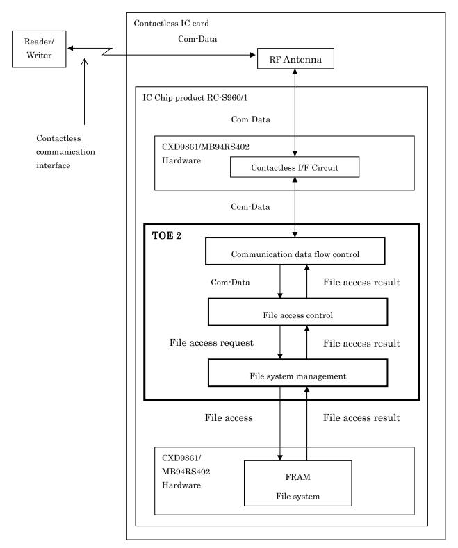
Figure 2-3 Functional configuration of the TOE 2
