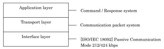
Application Layer: This layer defines the system of access to the file system, etc. of the TOE. TOE 2 is responsible for this layer.
