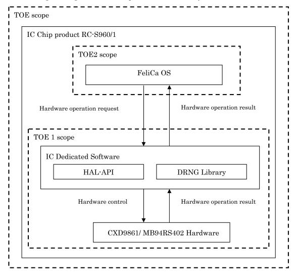
HAL: Hardware Abstraction Layer DRNG: Deterministic Random Number Generator HAL-API is a part of configuration of TOE1, and developed by the developer of TOE 1.
