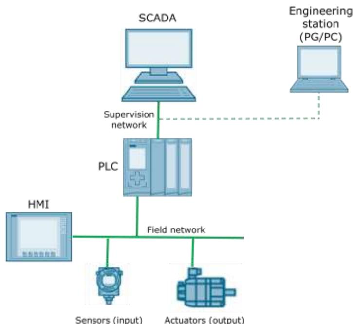
**Figure 2 - Typical network architecture for a PLC**
