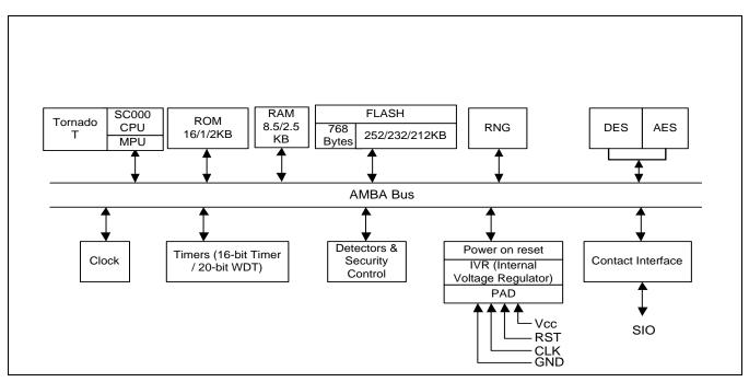
Figure 1 S3K250A/S3K232A/S3K212A Block Diagram
