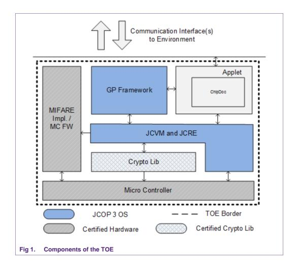
The TOE consists of an applet which is executed by a software stack that is stored on a Micro Controller. For a complete picture of the TOE see Figure 1, and for details with regards to the different components see section 1.3.1.
