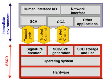
Figure 4 - Scope of the SSCD, structural view
