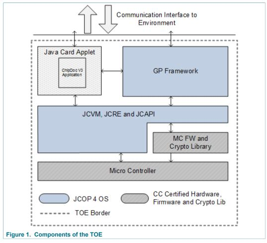
The TOE consists of an applet which is executed by a software stack that is stored on a Micro Controller. Figure 1 illustrates the components of the TOE, while Section 1.3.1 provides more details with respect to the dedicated components.
