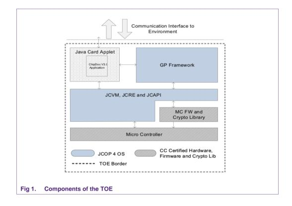
The TOE consists of an applet which is executed by a software stack that is stored on a Micro Controller. For a complete picture of the TOE see Figure 1, and for details with regards to the different components see section 1.3.1.
