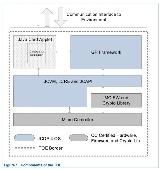
The TOE consists of an applet which is executed by a software stack that is stored on a Micro Controller. <u>Figure 1</u> illustrates the components of the TOE, while <u>Section 1.3.1</u> provides more details with respect to the dedicated components.
