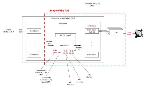
Figure 7 – TOE physical interfaces
