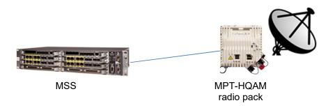
Figure 2 – 9500 Microwave Packet Radio (MPR) in Short Haul architecture
