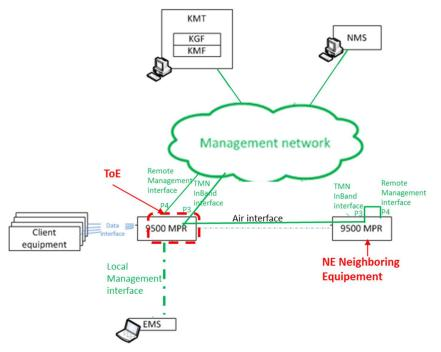
Figure 5 - System architecture alternative
