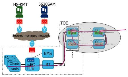
Figure 12 – 1+1 FD redundancy configuration
