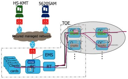
Figure 11 – 1+1 HSB redundancy configuration
