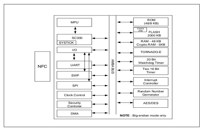
Figure 1 S3NSN4V Block Diagram
