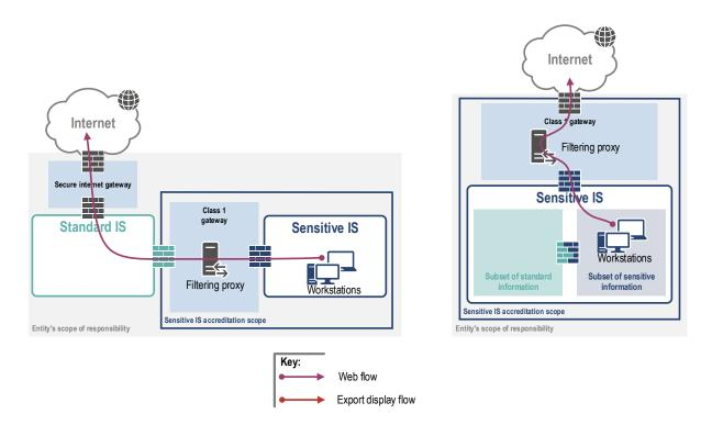
Figure 13 – Web browsing: example of an IS architecture of class 1, without bounce servers (left: case of a physically partitioned architecture; right: case of an architecture with logical partitioning of sensitive and standard information)
