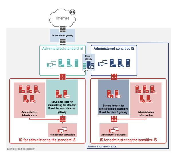
Figure 29 – Sensitive IS of class 1 - Positioning of the administration IS in the case of a "physically partitioned sensitive IS"
