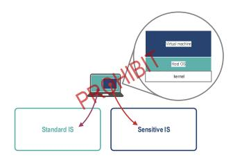
Figure 23 – Prohibited architecture: standard user workstation hosting a sensitive virtual machine
