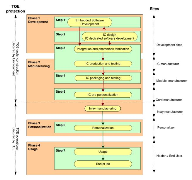
Figure 2: LC1: Pre-personalization on module at Gemalto site
