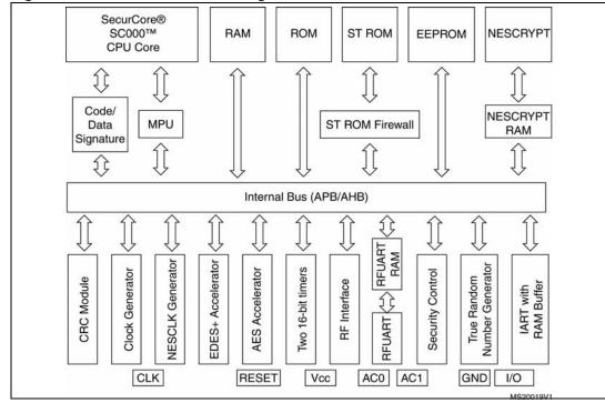
Figure 1. ST31 - K330A block diagram
