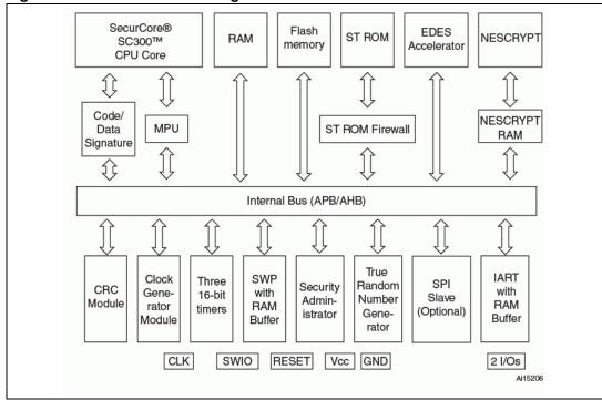
Figure 1. SM33Fxxx block diagram
