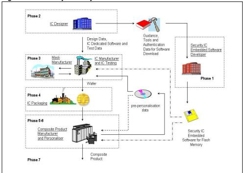
Figure 2. Security IC life cycle
