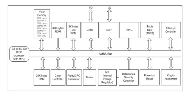
Figure 1: S3FS91J/S3FS91H/S3FS91V/S3FS93I Block Diagram
