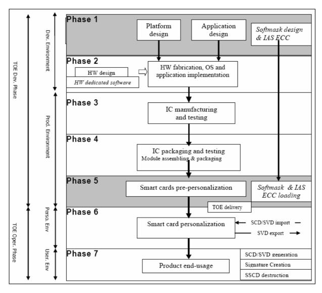
As show above, TOE delivery is done at the end of phase 5 (pre-personalization), after soft mask and applet loading.
