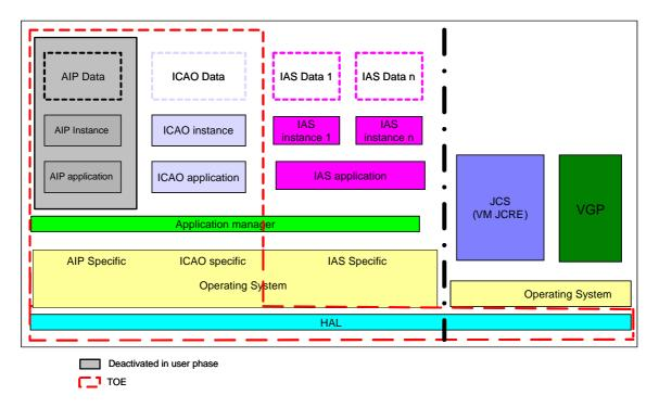
The TOE is the IAS Application, together with the functions/services provided by the operating system and the microcontroller IC required to support the applet functionalities.
