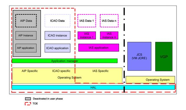
The TOE is the ICAO Application, together with the functions/services provided by the operating system and the microcontroller IC required to support the applet functionalities.
