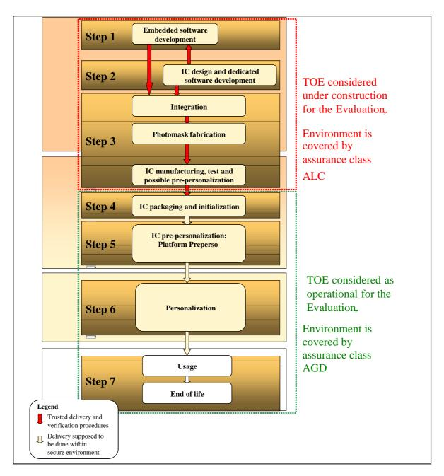
The evaluation has covered the conception and the development of the platform which are done in step 1. Steps 2 and 3, until delivery, have been covered by component evaluation. The end of step 3 and steps 4, 5 and 6 are covered by guides. The evaluated product is the one delivered to the user in step 7.
