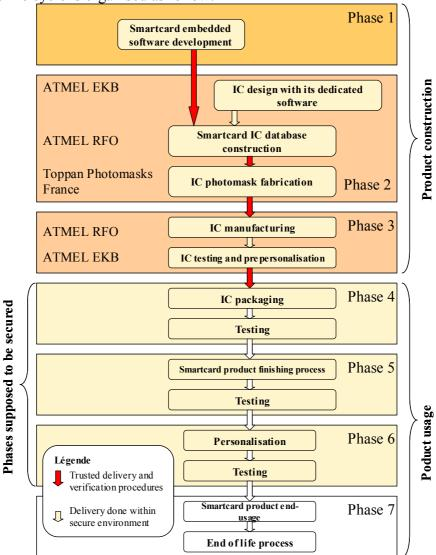
Figure 1 – standard IC life-cycle
