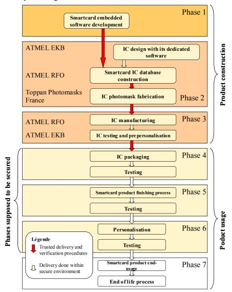
Figure 1 – standard IC life-cycle
