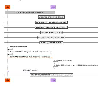
Figure 6: Security Function #4 - Secure Channel
