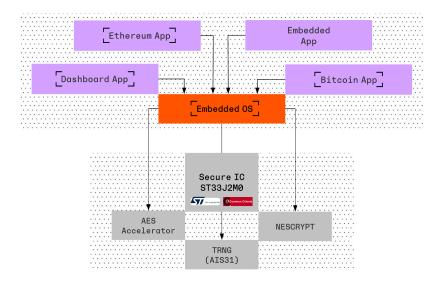
Figure 7: App Isolation on the Ledger Nano X
