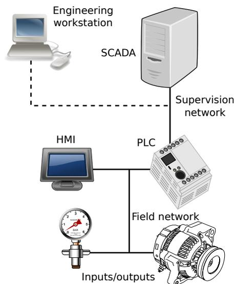
Figure 1: Typical network architecture for a PLC
