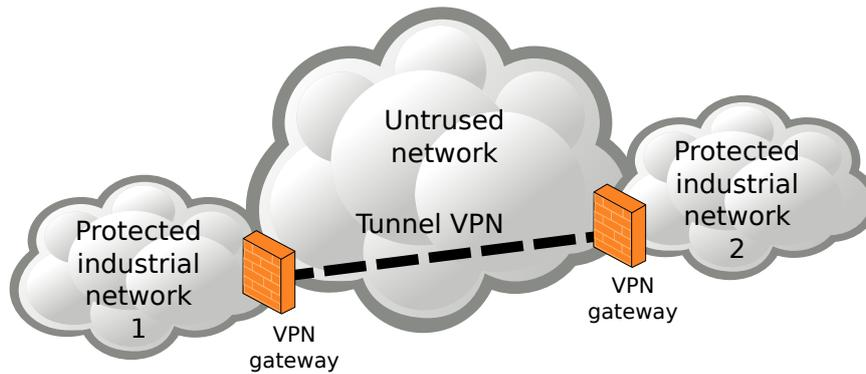
Figure 1: A VPN tunnel between two gateway
