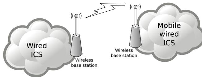
Figure 3: Wireless communication between to wired networks
