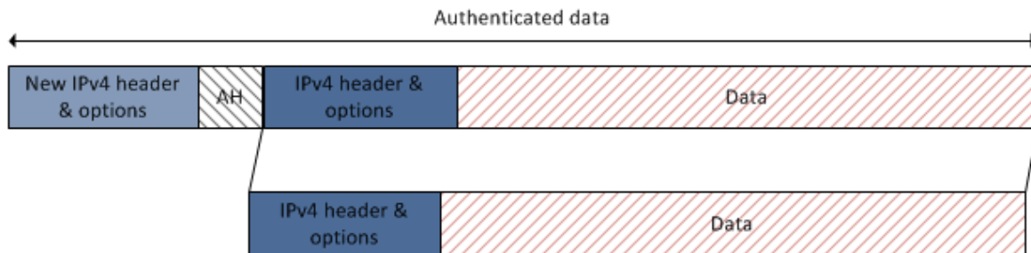
Figure 9: Using AH in tunnel mode. The ICV is included in the “AH” header
