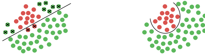
(a) Linear Model : does not fit well the training data. (b) Quadratic Model : fits well the training data.
